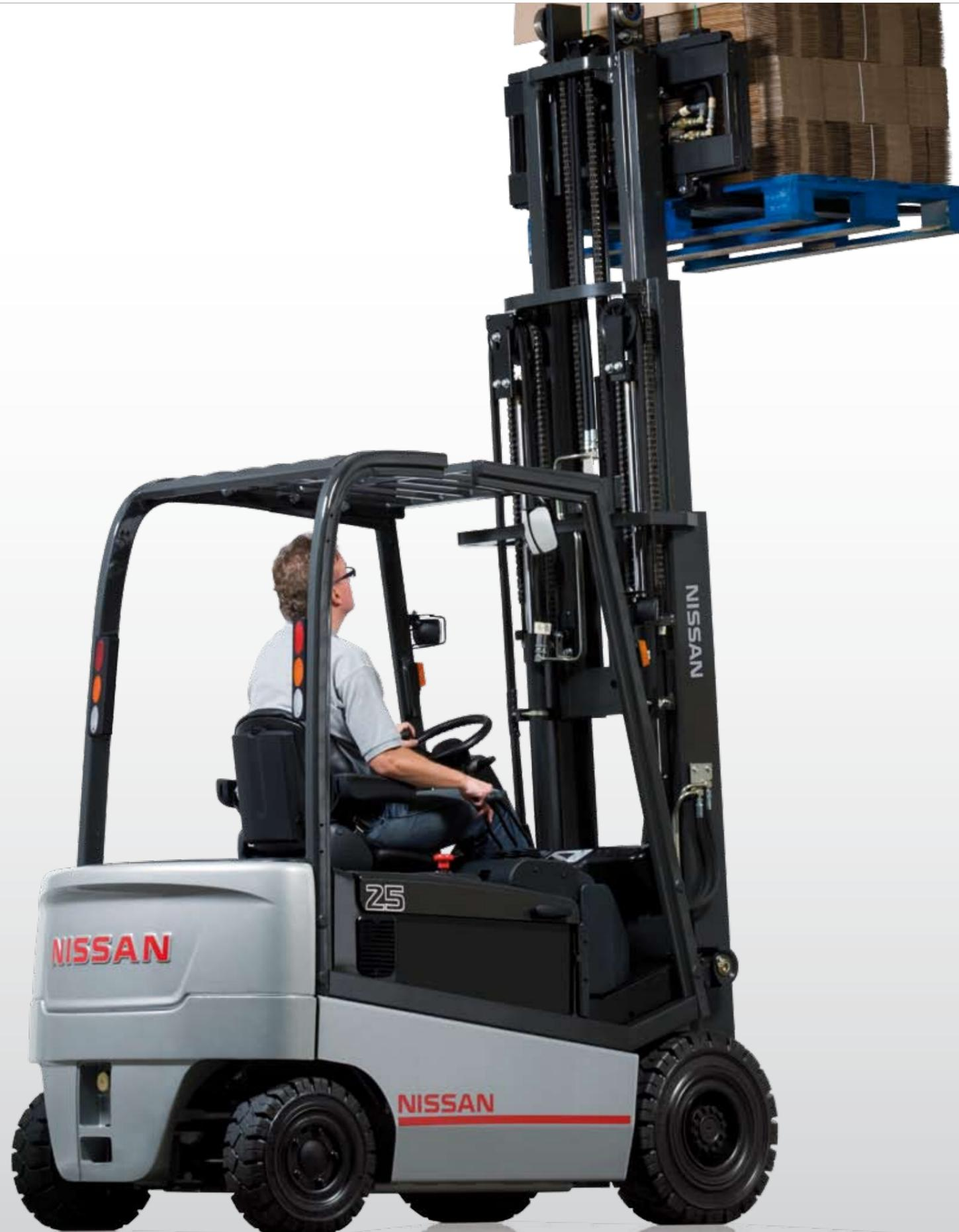
The Nissan QX2 Series has been designed and built to provide superior performance, whether the work requires rapid travel and lift speeds or slow speeds and precise control. Whatever it is that you need to handle, the AC TECH controller, regenerative braking systems, on demand power steering and Auto-Power Off function all ensure that the QX2 is one of the most productive and efficient forklifts in its class.
